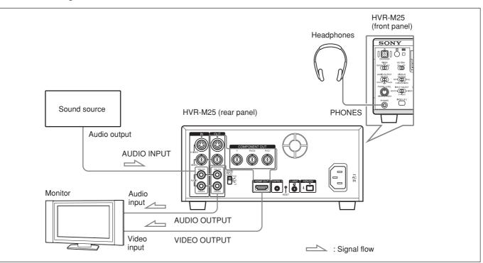
When an HDMI cable is used for connection, Audio cable connection is not necessary.
